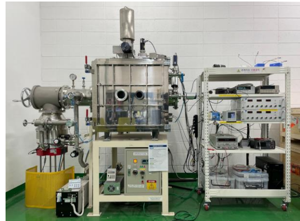
Fig. 2 An image of the laboratory vacuum chamber and measurement units. The chamber features a UV lamp for replicating solar radiation and a molecular pump for achieving high vacuum levels (less than 1\text{e-}7 mbar). The measurement units include vacuum gauge, electrometer, DC voltage supplier, etc.
