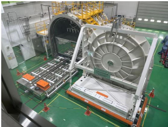
Fig. 1 An image of KICT's dirty thermal vacuum chamber (DTVC). The photograph shows the chamber, revealing a container holding artificial lunar regolith positioned inside the chamber.
